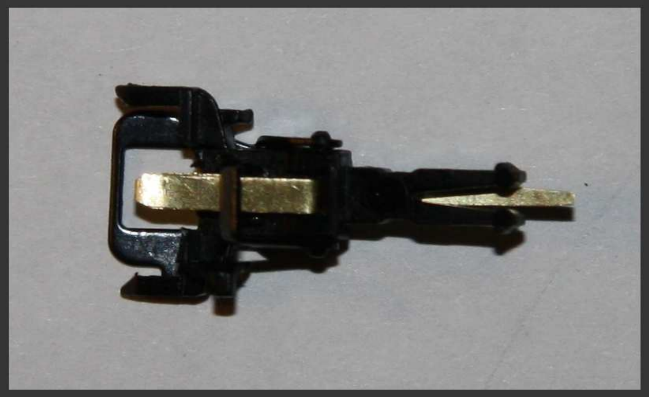
Detail of the hook seen from below.
